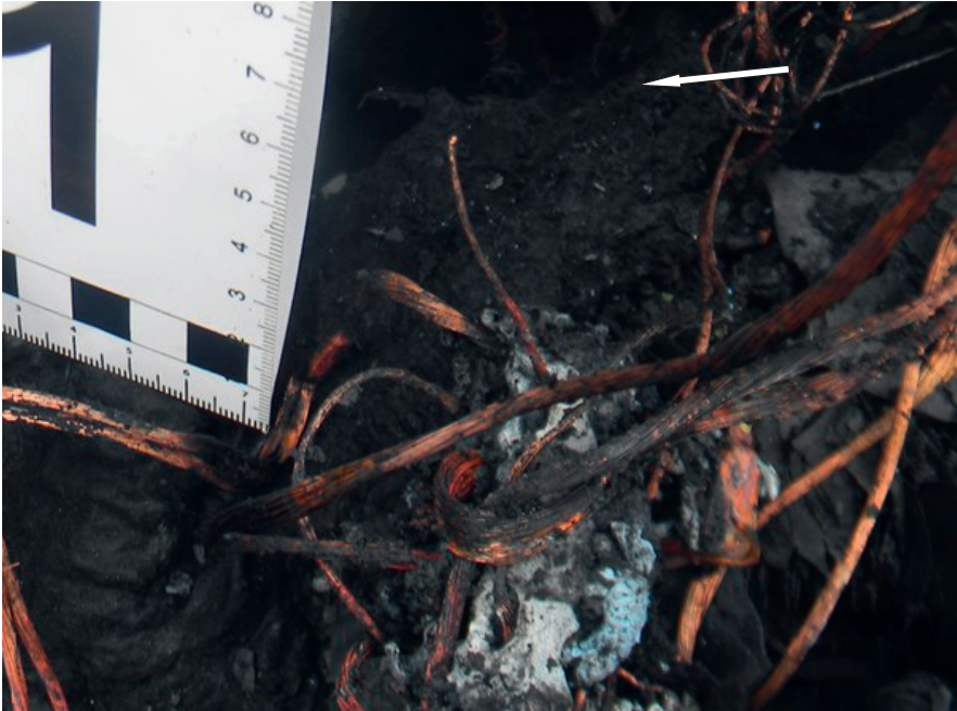
Photograph 5. The trace of a short circuit.
