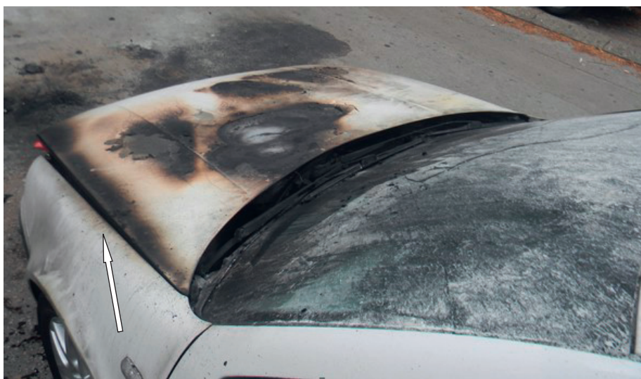
Photograph 4. Smoke halo on the edge of the hood.
